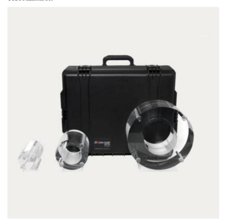
Adapt the size of the phantom RTI offers two different CTDI Phantom sets. Choose two (2) or three (3) parts. Both have nested modules to allow adaptation to the size required by the selected user protocol. [...]
